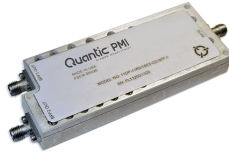
Low (10.75 to 12.25 GHz) / High (15.75 to 17.25 GHz) Diplexer
