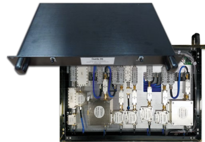
10 CH Switch Filter Bank
