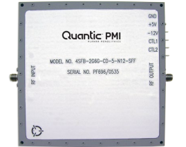
8 CH Switch Filter Bank
