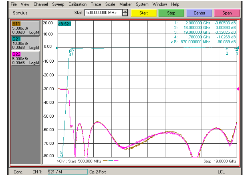
Insertion Loss & Return Loss (IN/OUT)
